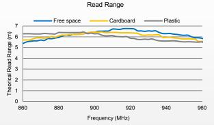
All the graphs are indicative: performance in real life applications may vary. The data has been determined based on calculations for transmitters with a 2W ERP output power level and an Impinj Monza R6-P tag silicon.
